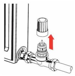
2. Press the sensor firmly onto the valve. Sensor horizontal: ensuring that the scale pointer is at the top. Sensor vertical: ensuring that the scale pointer is at the front.
