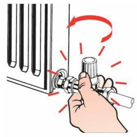
4. Remove the cap and turn the setting ring according to the drawings – the setting ring is turned by hand only.
