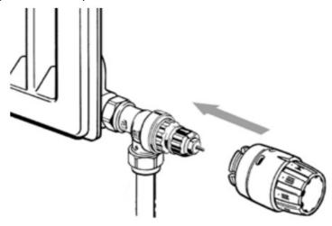
4. Whilst holding the sensor firmly on the valve secure connection by turning union nut clock-wise by hand.
