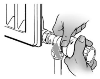
5. Whilst still holding the sensor firmly on the valve, tighten the grey union nut to 5Nm, using parrot nose pliers.
