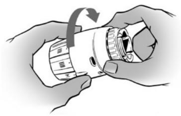
3. Press the sensor firmly onto the valve.
