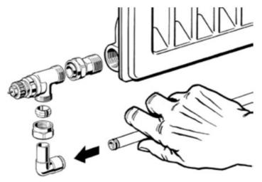
2. **IMPORTANT:** Both nuts have to be tightened It is good practice to check the fitting before use: pull the pipe back to check it is secure.
