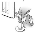
5. Whilst still holding the sensor firmly on the valve fully tighten grey union nut using parrot nose pliers.
