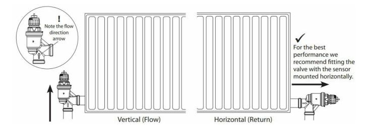
! If you are not installing a Danfoss lockshield valve (supplied in sets code, 013G7662 & 013G7663) ensure that the lockshield is fully open. No balancing on the lockshield/return pipe.
