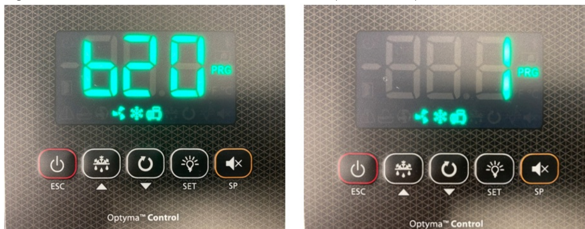
Fig. 6: Parameter “b21” set to 1, for baud rate 19200
