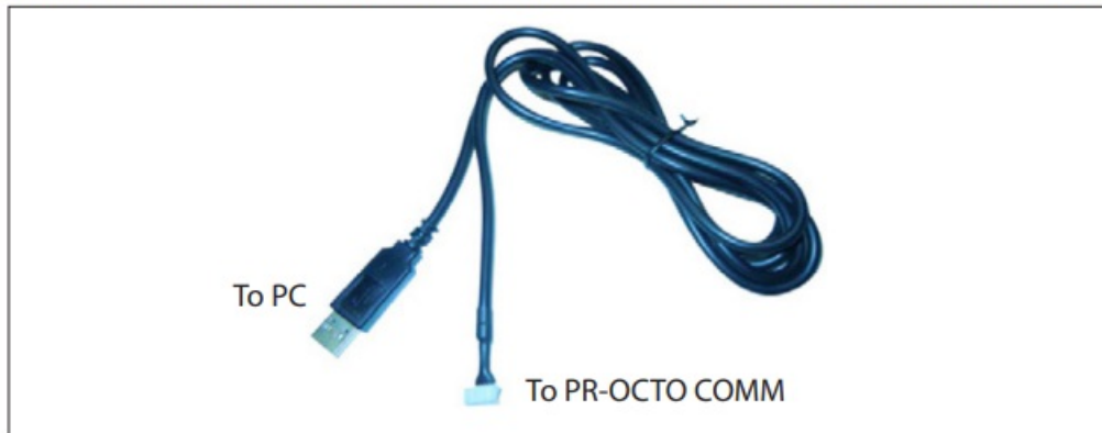
Fig. 5: PC Test Cable for monitoring the PR-OCTO GPRS transmission signal level.
