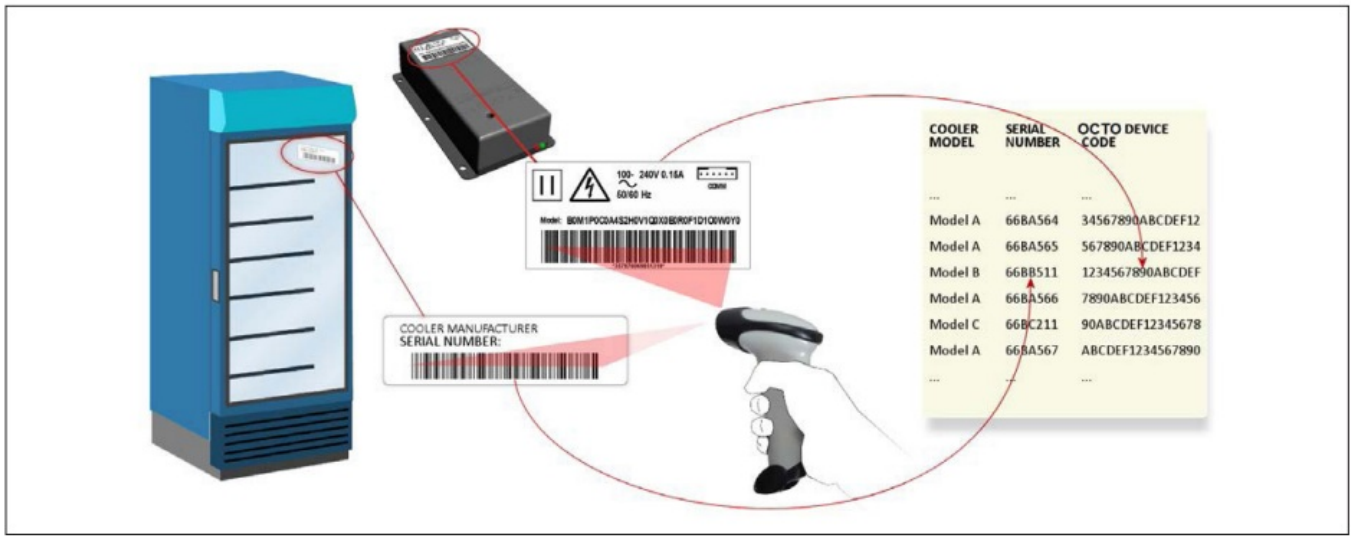
Fig. 8: Association between PR-OCTO device and the specific cooler.
