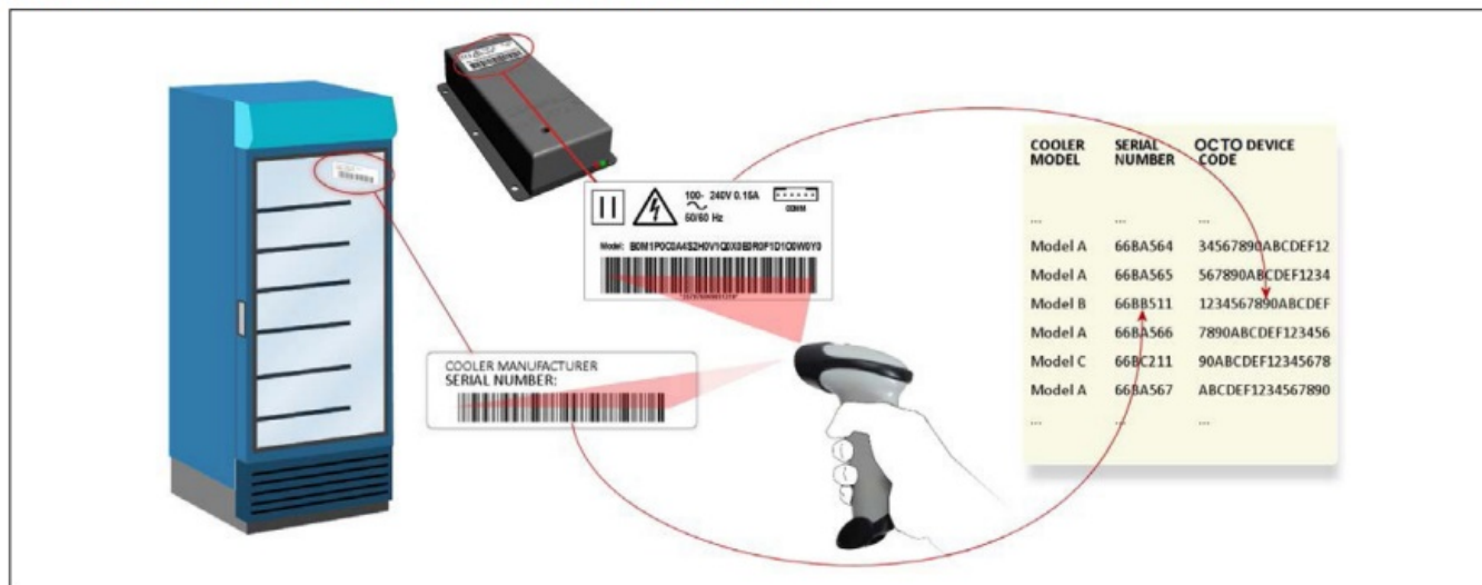
Fig. 8: Association between OCTO device and the specific cooler.
