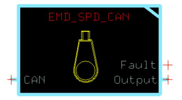
This function block outputs an RPM signal and a DIR signal based on inputs from an EMD Speed Sensor. All signals are received via the CAN communication bus.
