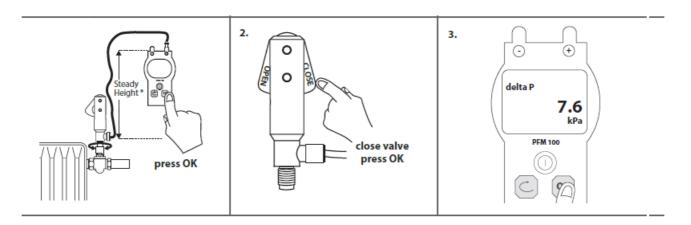
Pump Optimization with the Danfoss Δp Tool for Dynamic Valve™ (example)
