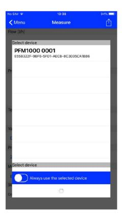
You can cancel the Always use the selected device from the Application Setup, the Sensor Preferences / Always use Bluetooth Address option. Here, delete the Bluetooth address of your pressure unit module.
