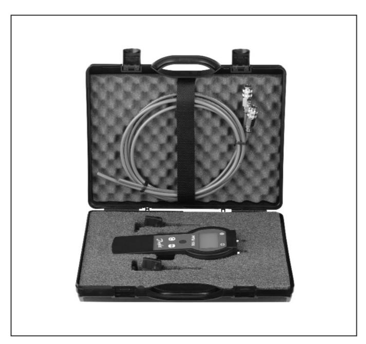
The PFM 100 is used for measuring the differential pressure on both sides of a valve in hydronic systems.
