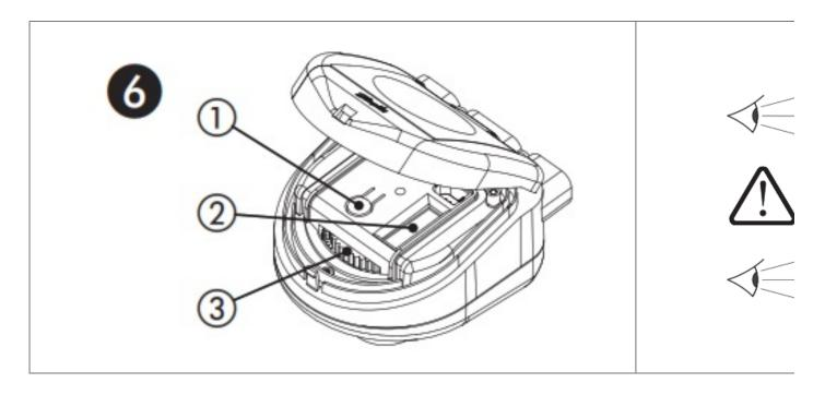
Manuel Calibration: Press button ① until two LEDs are turned on, and then release again. DIP switch: ② Manual override: Adjust wheel ③
