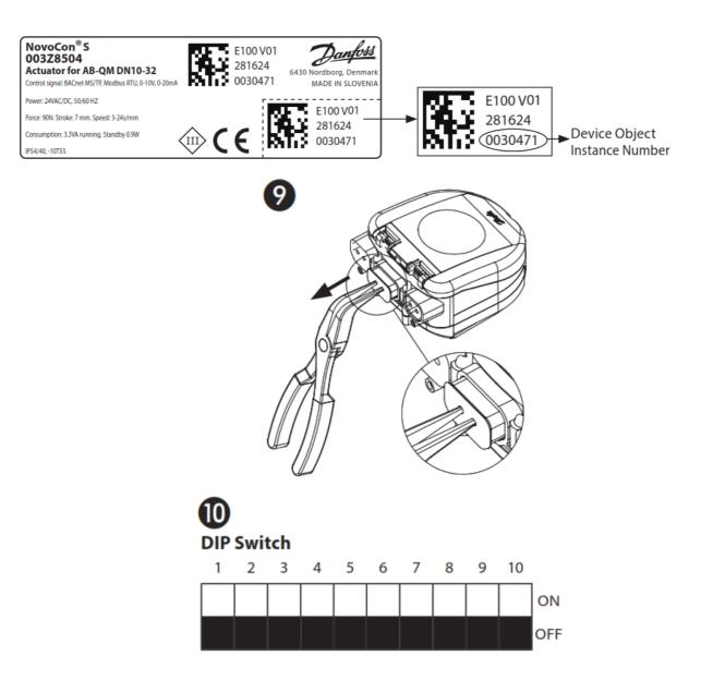
DIP Switches 1 to 7 is used to assign the MAC address manually.
