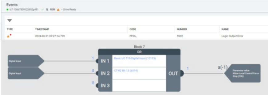
Illustration 4: Logic output error event because -1 is not a valid choice for parameter number 106
