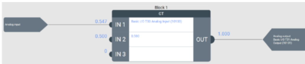
Illustration 2 : Live debugging values shown on the inputs and outputs of a (Greater Than(GT) Function block
