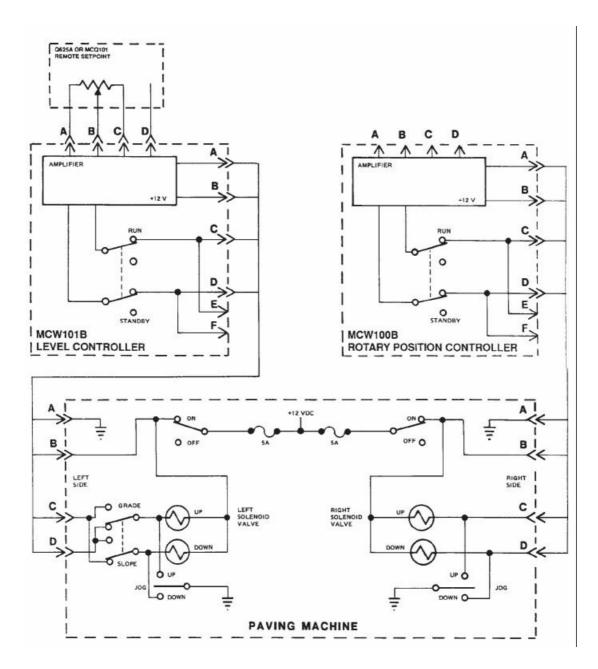
Typical Wiring Diagram for the MCW101A Level and MCW100A Rotary Position Control. Level and Rotary Position Controllers May Be Interchanged.
