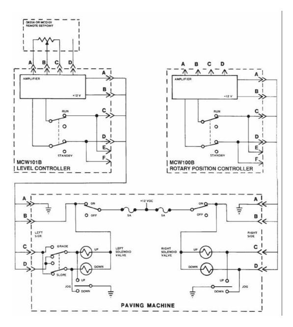
Typical Wiring Diagram for the MCW101B Level and MCW100B Rotary Position Control. Level and Rotary Position Controllers May Be Interchanged.
