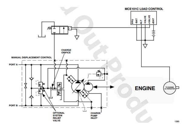
MCE101C Used in a Closed-loop Load Control System.
