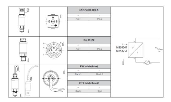
Cables must be specified for a minimum test voltage of 500 VAC between conductor/earth, conductor/screen and screen/earth.
