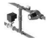
Make sure that the surface of the pipe is clean and even where the sensor is mounted.
