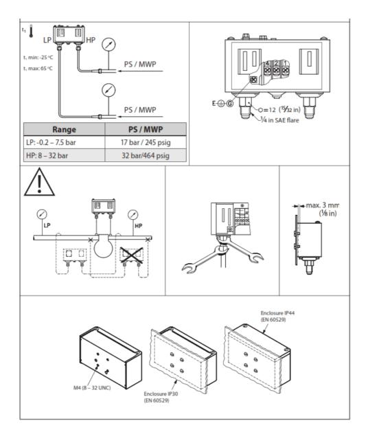
**CAUTION:** Disconnect the power supply before wiring connections are made or serviced to avoid possible electrical shock or damage to equipment.
