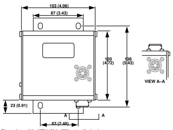
Dimensions of the KE04109 in Millimeters (Inches).
