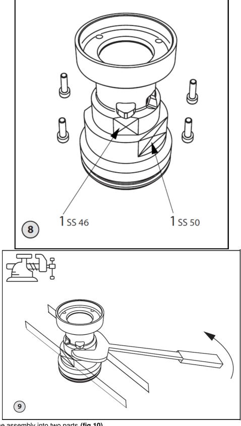
3. Disassemble the assembly into two parts (fig 10)
