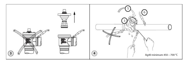
The top cover, complete with the function module, should be removed before welding or brazing to prevent
