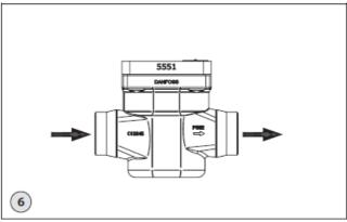
The valve must be installed with the arrow in the direction of the flow and the top cover upwards (fig. 1 and 6). The top cover can be rotated 4 X 90° in relation to the valve body. The valve is designed to withstand a high internal pressure. However, the piping system should be designed to avoid liquid traps and reduce the risk of hydraulic pressure caused by thermal expansion. It must be ensured that the valve is protected from pressure transients like "liquid hammer" in the system.
