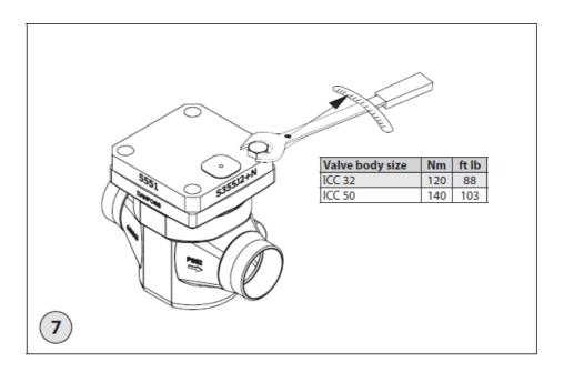
Tighten the top cover with a torque wrench, to the values indicated in the table.
