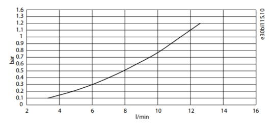
Illustration 10: Pressure Drop, L Filter OF7Z5, 690 V/400 A
