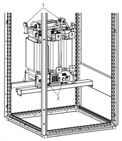
Illustration 4: Installing the L Filter into a Cabinet (400 A, 1000 A)
