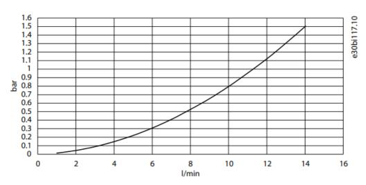
Illustration 11: Pressure Drop, L Filter OF7Z5, 690 V/1000 A
