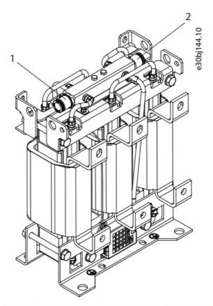
Illustration 13: Inlet and Outlet Connectors of the L Filter
