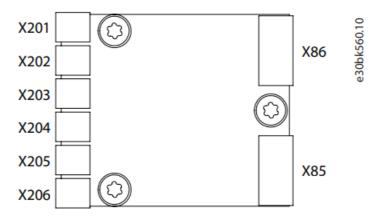
Illustration 16: Terminals on the AuxBus Temperature Measurement Board
