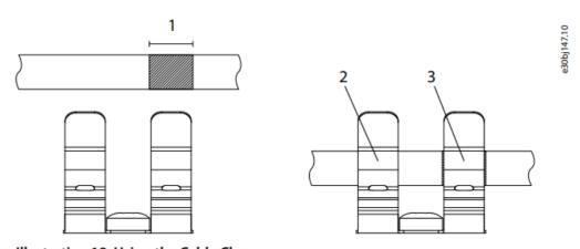
Illustration 18: Using the Cable Clamps
