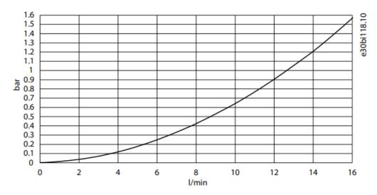
Illustration 12: Pressure Drop, L Filter OF7Z5, 690 V/1640 A
