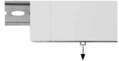
3. Release from DIN-rail.
