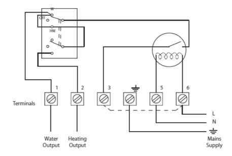
**NOTE:** Terminals 3 and 6 MUST be linked externally (except when voltage-free switch contacts are required).
