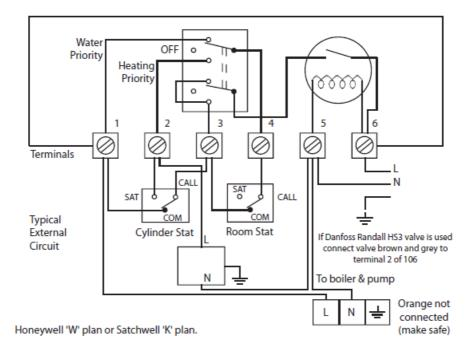
Fully pumped system with 3 port (2 way) diverter valve.
