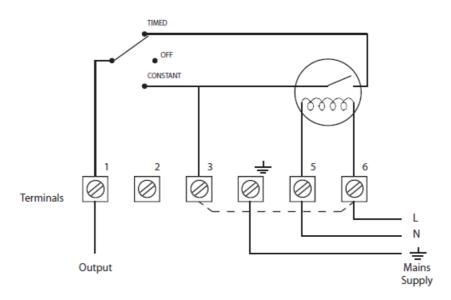
**NOTE:** Terminals 3 and 6 should (in most instances) be linked externally. Exceptions are when control circuits are operating at low voltage (e.g. 24 volts) or for certain Combination Type Boilers (see Boiler Manufacturers Handbook).
