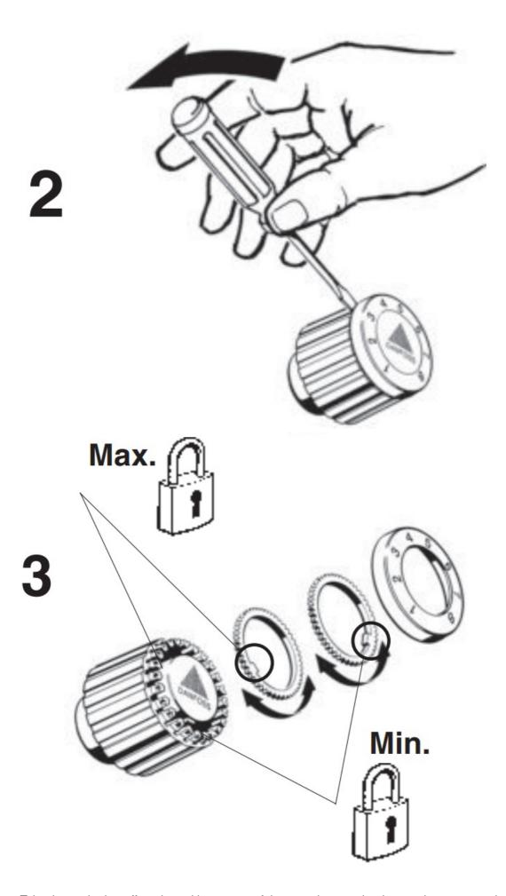
Take the scale ring off again and insert one of the stop rings so that its stop lug contacts the righthand side of the lug on the centre piece (fig. 3). Place the scale ring in position with »2« opposite the arrow.
