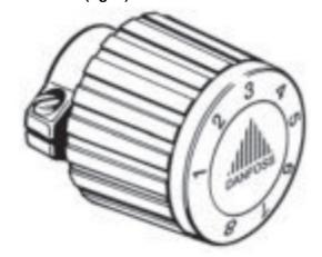
Remove the scale ring with a screwdriver (fig. 2). Take the two stop rings out of the selector knob gear rim (fig. 3). Place the scale ring as shown in fig. 1 and set the knob to the required minimum value, "2" for example.
