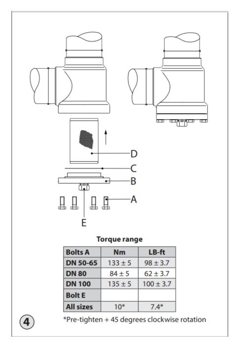
Before servicing the strainer, isolate it from the system. Drain  $CO_2$  e.g. via the top cover connection to above 5,2 bara to prevent large formation of dry ice before evacuation to zero pressure. Check for refrigerant pressure before unscrewing and removing the top cover. The strainer insert must be removed without any use of tools.
