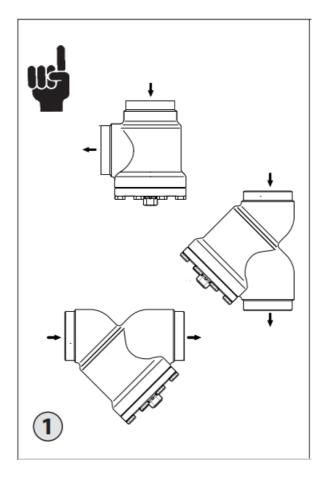
The strainer housing is designed to withstand a high internal pressure. However, the piping system should be designed to avoid liquid traps and reduce the risk of hydraulic pressure caused by thermal expansion. It must be ensured that the strainer is protected from pressure transients like "liquid hammer" in the system.
