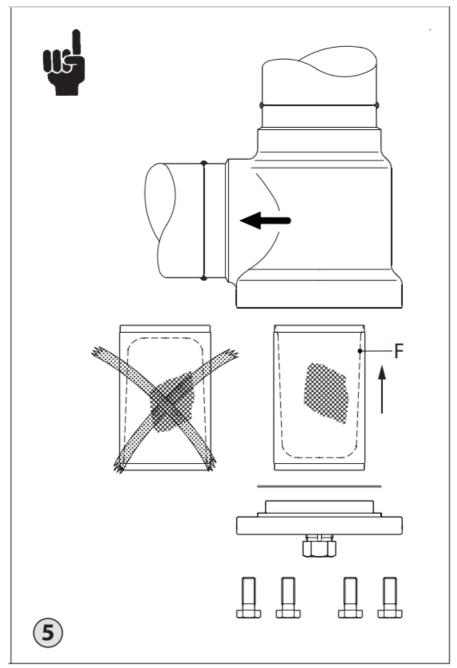
The flow must go into the filter bag cavity and out or else the bag will not function properly.
