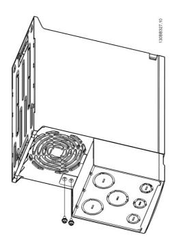
**Step 2**Fit bottom cover on drive and tighten screw.
