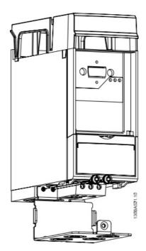
**Step 4**Fit bottom cover on drive and tighten screw.
