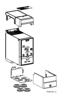
**Step 3**Mount metal plate on drive and tighten screws.
