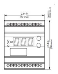
Mounting: DIN rail Enclosure: IP 20
