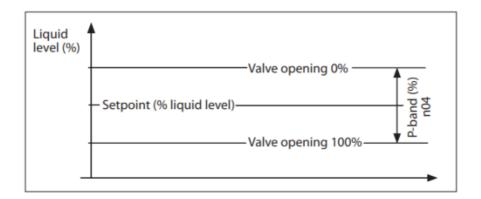
Regulation example 1. Valve opening percentage will modulate to maintain the setpoint liquid level percentage. The P-band defines the liquid level percentage range allowed.
