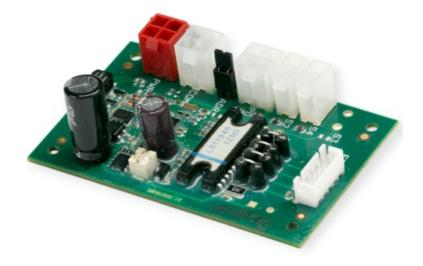
The EIM 336 is the superheat controller that can be used to control the opening degree of a valve based on the superheat of the evaporator. This is applicable in applications such as air conditioning, heat pumps and refrigeration. An alternative option is to use the controller in manual mode via modbus communication and use it as a valve driver by setting the valve opening degree manually.
