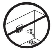
• Do not place the thermostat on the inner side of an exterior wall.
