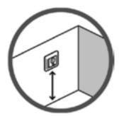
• The thermostat should not be placed in wet rooms. Place it in an adjacent room. Always place the thermostat according to local regulation on IP classes.
