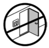
• Do not place the thermostat in a way that it will be exposed to direct sunlight.
