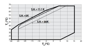
The compressor must only be used for its designed purpose(s) and within its scope of application (refer to "operating limits"). Consult Application guidelines and datasheet available from cc.danfoss.com Under all circumstances, the EN378 (or other applicable local safety regulation) requirements must be fulfilled. The compressor is delivered under nitrogen gas pressure (between 0.3 and 0.7 bar) and hence cannot be connected as is; refer to the "assembly" section for further details.
