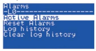
Active alarms: display of the currently active alarms and is to navigate like Alarm view. Having an active alarm will activate alarm relay. Alarms will be retained till reset has been performed.
