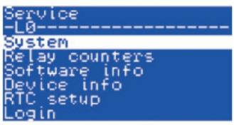
**System:** contains a system submenu for professional users containing (Yxx) parameters.
