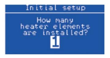
The device will now ask for the details of each heater in the following pattern
