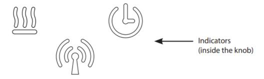
All indicators fade out after a duration (default 20 seconds) unless an error is present. Additionally, indicators will "wake up" upon manual interaction with the thermostat, heating state change, schedule event, app connection or errors/warnings appearing.
