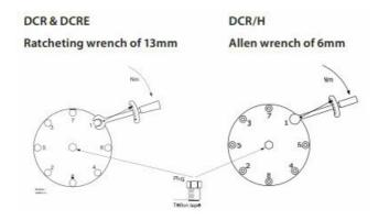
Optional Plug, recommended tightening torque: Plug: 1/4" NPT: 50 Nm / 36.87 ft-lb applying 2 to 3 wraps of teflon tape.
