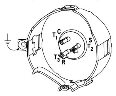
• Ring connect screw terminals C & Q terminal box type
