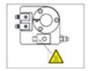
Before restart of compressors after a long period of standstill the oil level has to be checked on the sight glass
