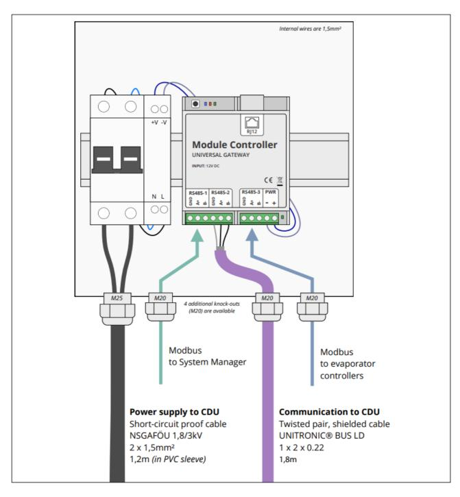
Connect Module controller power supply cable to L1 (left terminal) and N (right terminal) of the condensing unit control panel – power supply terminal block
