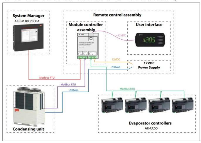
Power supply to CDU 230V AC 1,2m cable for this is included.
