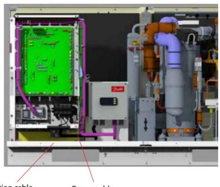
The communication cable and the power cable should not touch the baseplate
