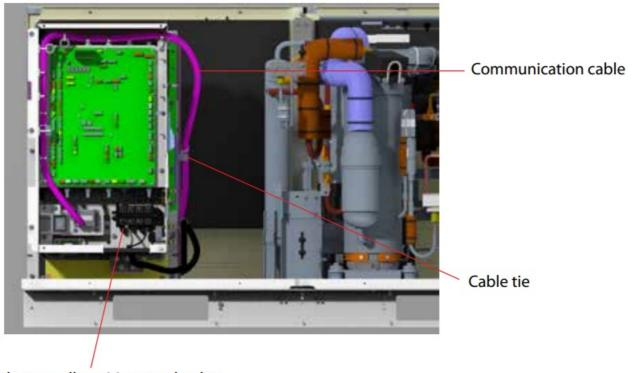
Module controller wiring need to be connected to the L1 and N -Terminals
