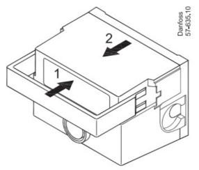
A front plate with knockouts or a front plate designed for PG 11 screwed connections can be used.
