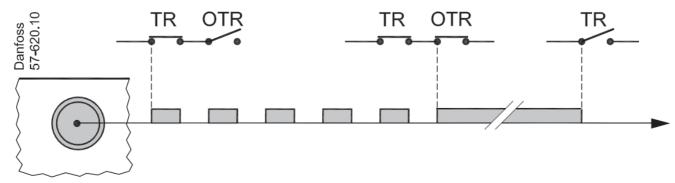
When the boiler thermostat cuts out, the green light turns off. On the OBC 85, the light does not turn off until the post-purge period ends.
