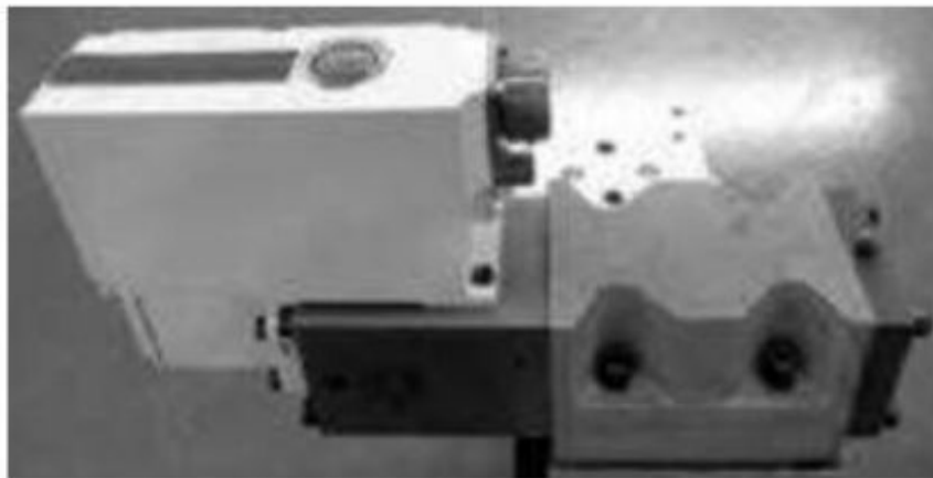
Figure 5. Mount the AxisPro valve to the adaptor plate.
