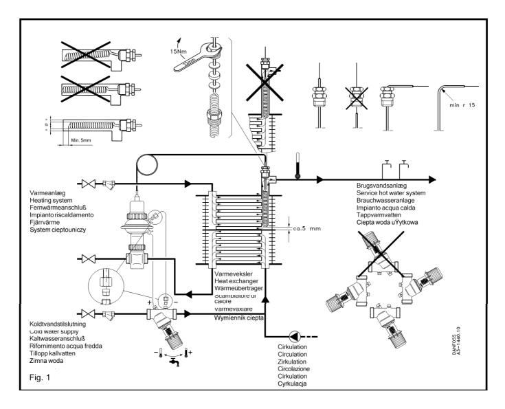
For correct no-load function, the thermal flow should be avoided as the hot water will rise and thus increase the no-load consumption. For optimum orientation of pressure connections loosen the nut (1), turn the diaphragm part into the desired position (2) and tighten the nut (20 Nm) – see fig. 4.
