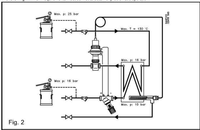
Before setting, the system should be flushed and vented, both on the primary side and secondary side of the heat exchanger. The capillary tubes from the pilot valve to the diaphragm should also be vented on the (+) as well as the (-) side.
