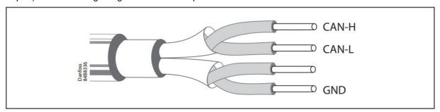
• The line termination must be present on both bus ends to ensure proper communication.
