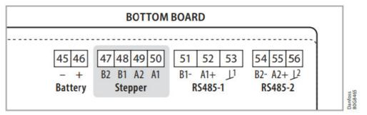
Valve cable connection Maximum cable length: 30 m
