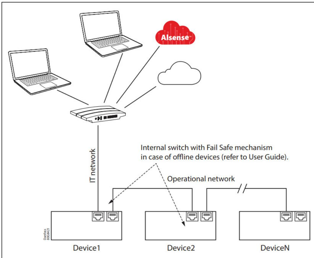
Point to point star topology with network hubs/switches. Each AS-CX device incorporates a switch with fail-safe technology.
