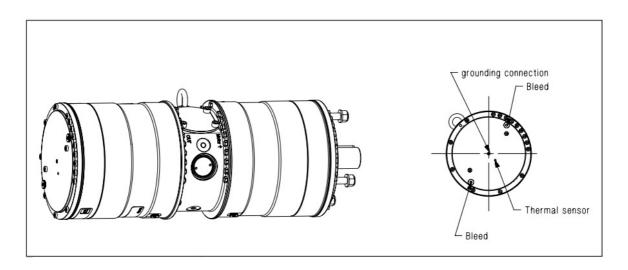
To prevent stray current corrosion we recommend grounding of the pump and all other parts in the system. All parts in the system must be electrical potential equalized to a single reference point (grounding point). It is recommended that the electrical resistance in the grounding cable is equal to or below 0.25 Ohm toward the grounding point.
