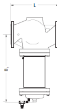
VFG, VFGS DN 150-250 with body extension
