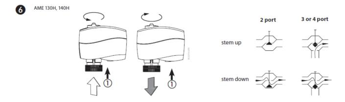
**Remark:** A 'click' sound after energising the actuator means that the gear wheel has jumped into normal position.
