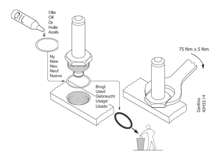
The gasket must be exchanged, if the valve is dismantled
