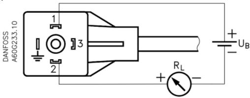
0-5 V, 1-6 V, 0-10 V d.c. output, ratiometric 10 – 90% V supply
