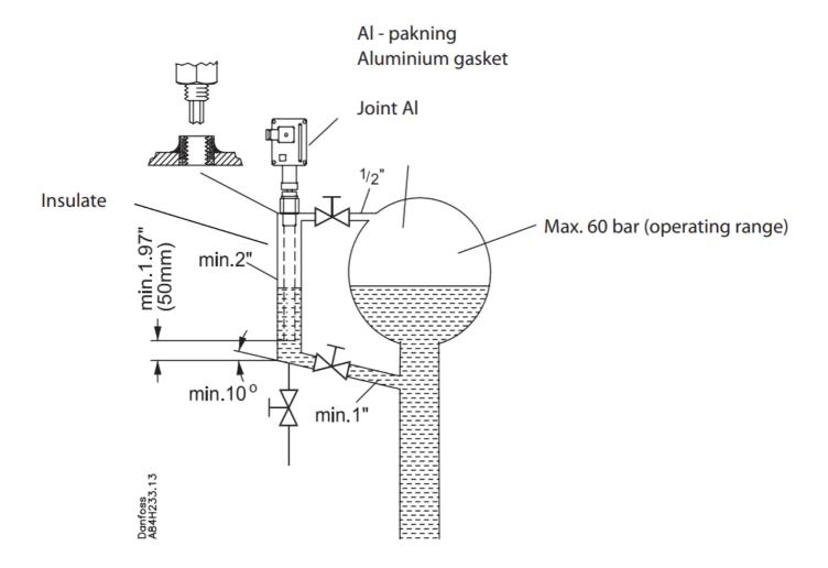
Remember clearance required for replacement of level transmitter, if applicable
