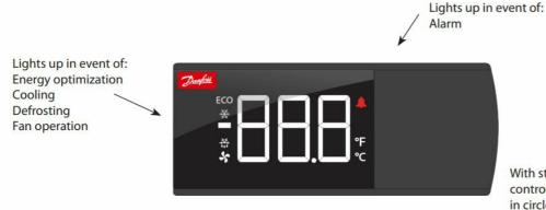
With start-up /connection to a controller, the display will "light up in circles" as it collects data from the controller.
